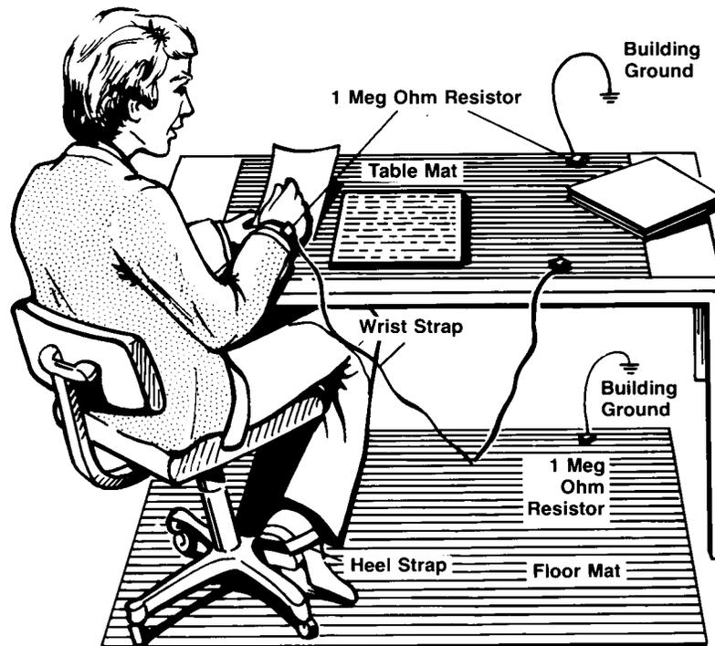
Both types, when used together, provide a significant level of ESD protection. Of the two, only the table-mat and wrist-strap combination provides adequate ESD protection when used alone. To ensure user safety, the static-safe accessories must provide at least 1 M $\Omega$  of isolation from ground. Purchase acceptable ESD accessories from your local supplier.
