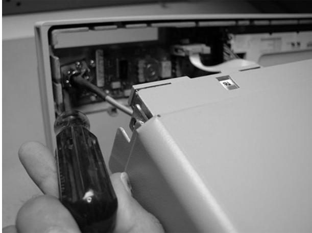
**Figure 7-9. Removing Screws that Secure the Cal Connector**
