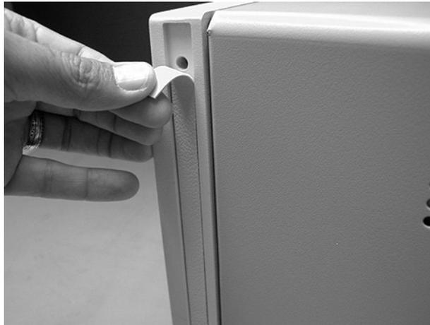
**Figure 7-27. Removing the Trim Strips**
