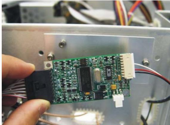
**Figure 6-7. Mount the Touch Screen Controller Assembly**
