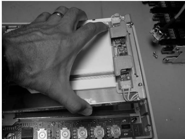
**Figure 7-26. Removing the Display**
