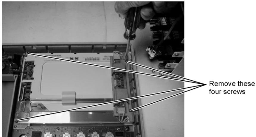
**Figure 7-25. Removing the Display Screws**
