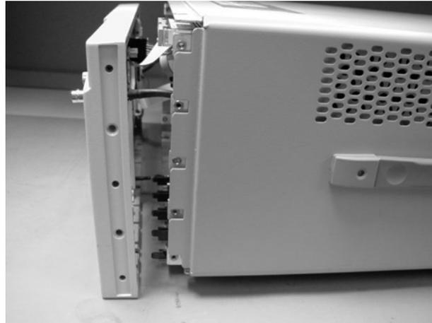
**Figure 7-8. Sliding Front Panel Away From Mainframe**
