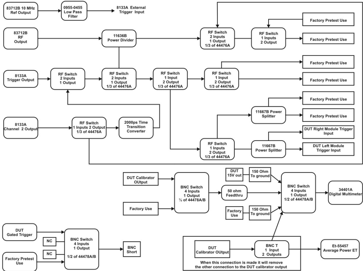
Figure 2-3. Test System Block
