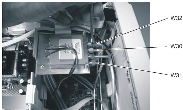
**Figure 7-60. Removing the Cables from SW2 Transfer Switch**
