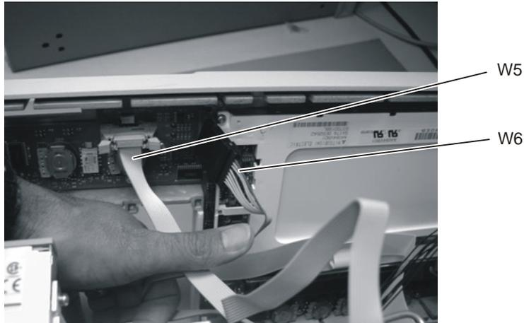
**Figure 7-10. Removing the W5 and W6 Ribbon Cables**
