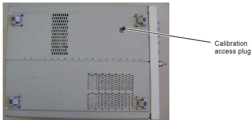
**Figure 6-4. Calibration Access Plug**
