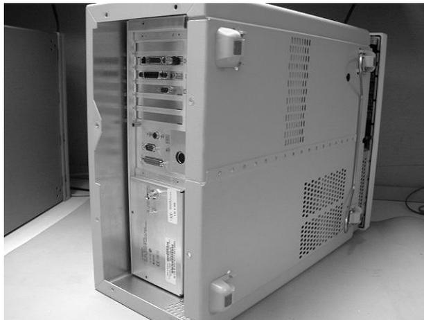
**Figure 7-5. Sliding Cover off Mainframe**
