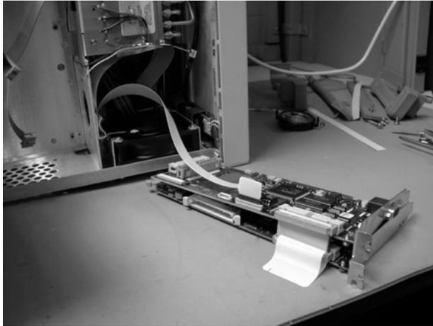
**Figure 7-35. Removing the A5 and A6 Boards**
