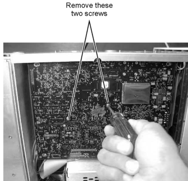
**Figure 7-62. Removing the A13 Acquisition Board Screws**
