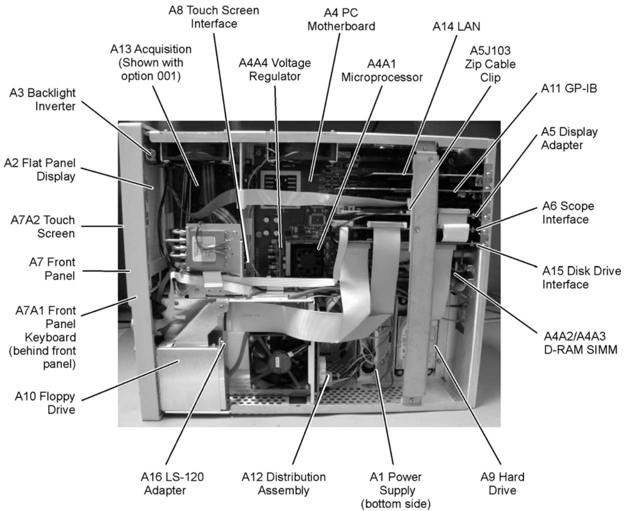
Figure 8-1. 86100A Major Assembly and Cable Location
