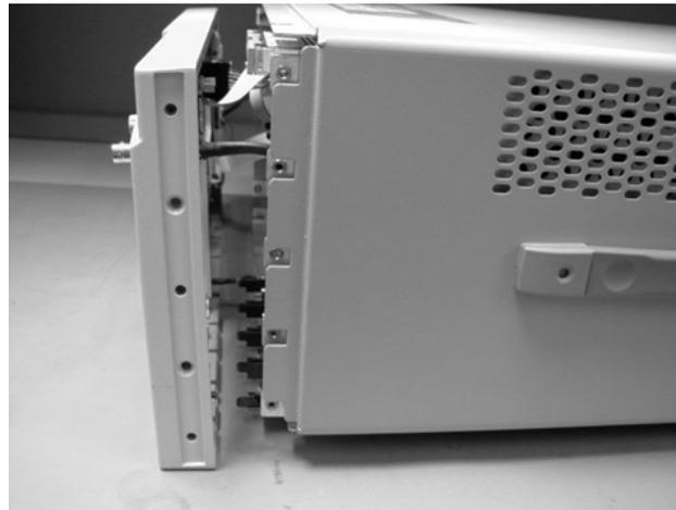
**Figure 7-16. Slide Front Panel Away From Mainframe**
