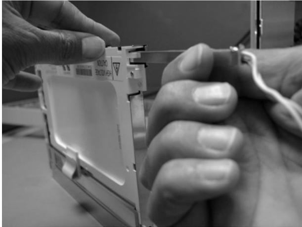
**Figure 7-19. Removing the Backlight**
