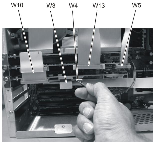
**Figure 7-45. W3, W4, W5, W10, and W13 Cables**
