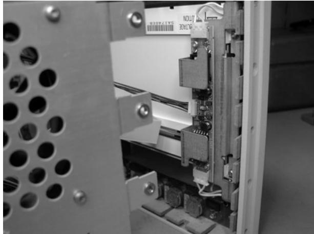
**Figure 7-29. Accessing the Inverter Board**
