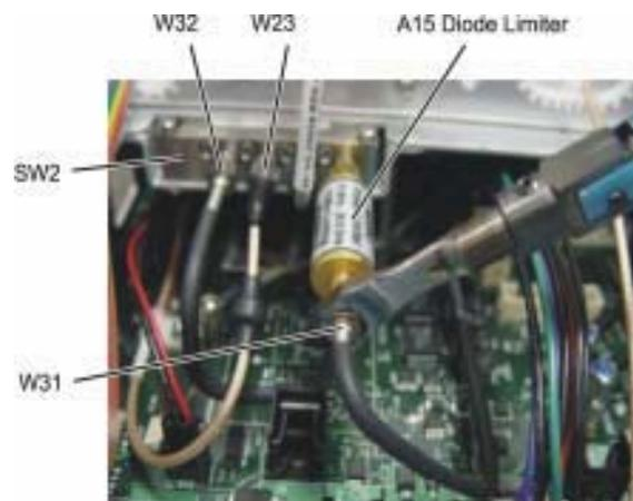
**Figure 7-61. A15 Diode Limiter on 86100C Option 001 instrument**
