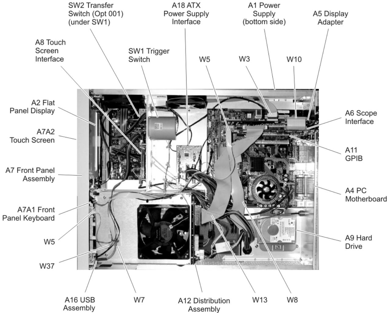
**Figure 10-1. 86100C Major Assembly and Cable Location**
