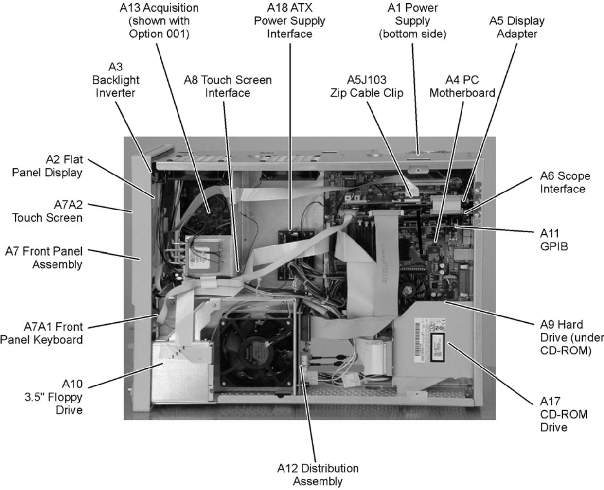
**Figure 9-1. 86100B Major Assembly and Cable Location**
